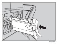
Remove the red sheet from the PCU, and then remove the two strips of tape.
